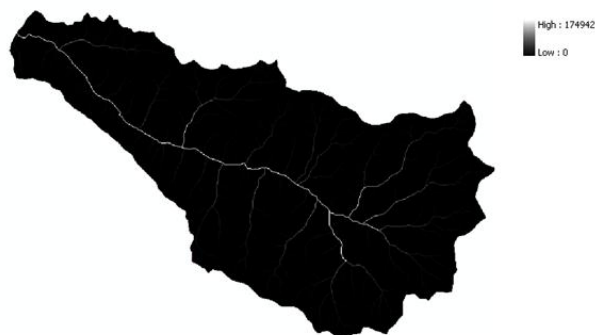
Fig. 6 Flow accumulation in the River Banjska basin up to the “Vranjska Banja” HS
