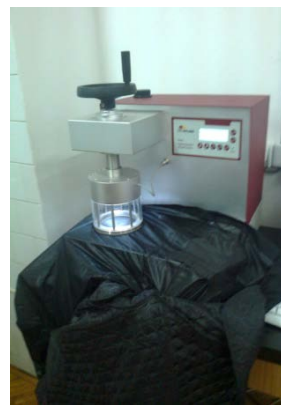
Figure 3. Determination of resistance to water penetration on the hydrostatic pressure tester according to the ISO 811 standard [6]
