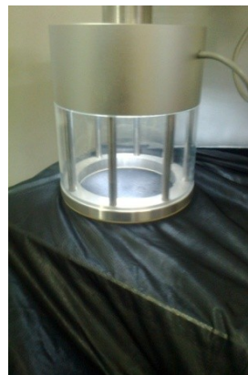
Figure 3. Determination of resistance to water penetration on the hydrostatic pressure tester according to the ISO 811 standard [6]
