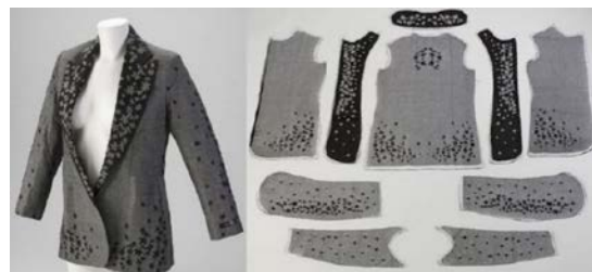
Figure 8. Garments and cuts produced by DPOL technology
