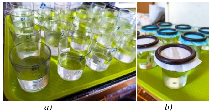
Figure 2. Water vapour permeability measurement: a) sample cup, b) open cup
