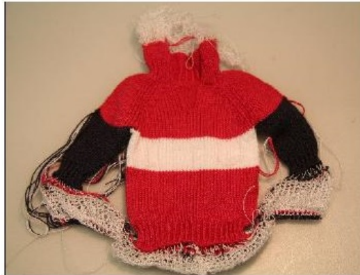
Figure 7. Seamless product – integral knitting
