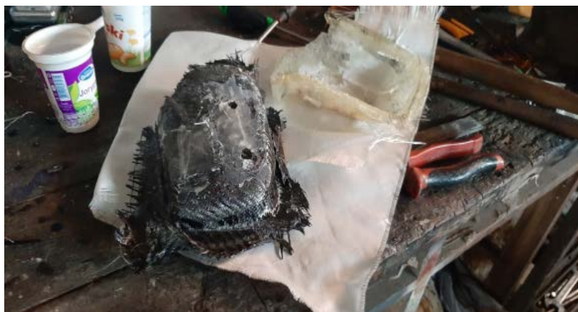
Figure 3: Appearance of the carbon part I of the mold after separation
