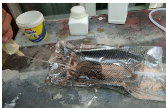
Figure 6: Appearance of creating a vacuum in a bag (Nylon) using a vacuum pump
