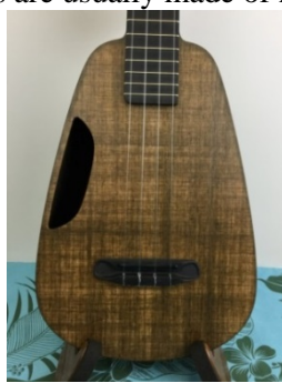
Figure 9. Linen Fiber Composite Ukulele [15]
