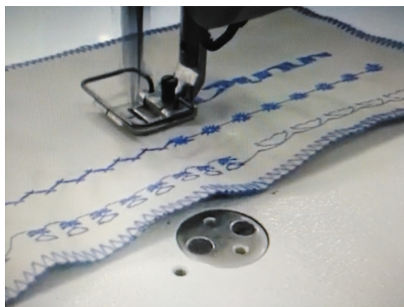
Figure 4. Decorative stitches created with needle movement left - right and forwards- backwards using stepping motors
