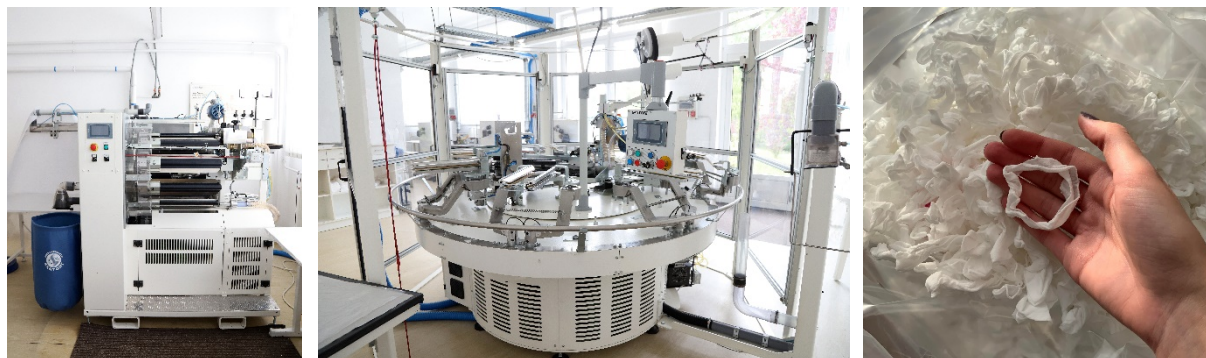
Figure 2. Hosiery machinery and the waste generated during the production (right)
