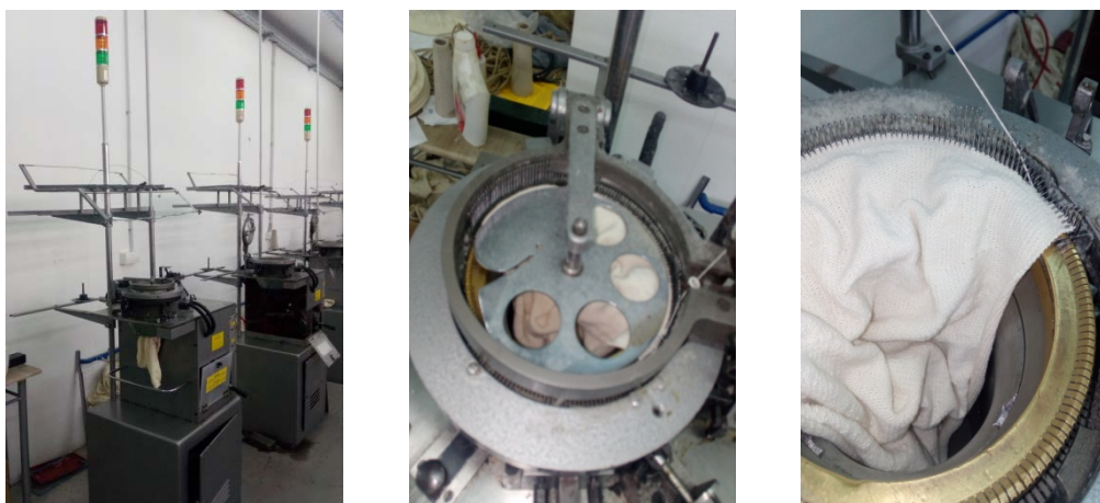
Figures 3,4,5: Beret production process on knitting machines
