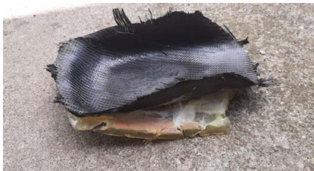
Figure 4: Appearance of carbon fiber and mold with lard as a pre-war material – front
