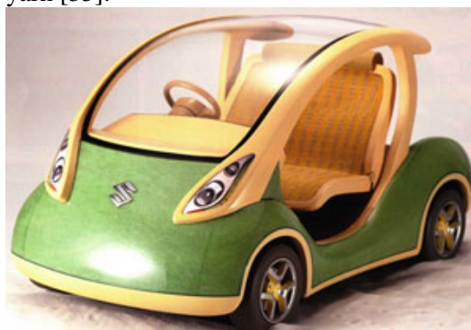
Fig. 2 Car made from banana fiber (Concept EV- SUZUKI) [35]
