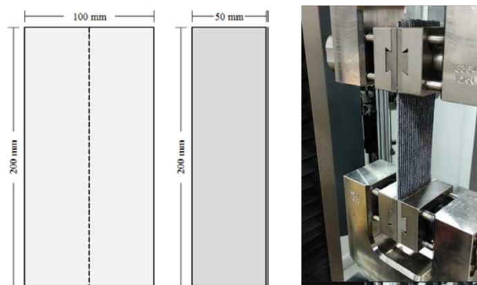
Figure 2. The elongation and tensile test sample (fabric opened and folded) and test device
