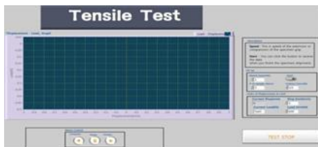
Figure 3: The user interface written in LabVIEW. The interface includes a real-time plot of the applied load against displacement. Also included are setup routines for the sample setup process
