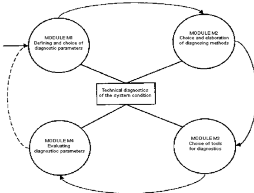
Figure 3: Modules of technical diagnostics within the process of the maintenance according to the condition
