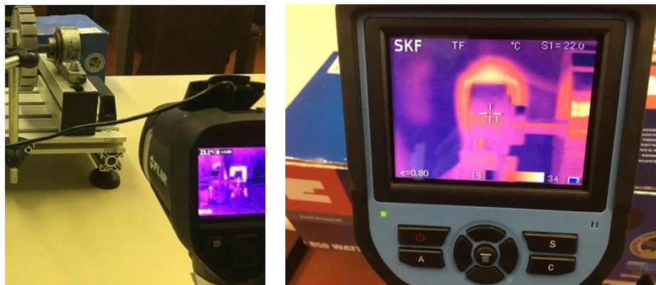
Figure 5. IR camera screen during measurement
