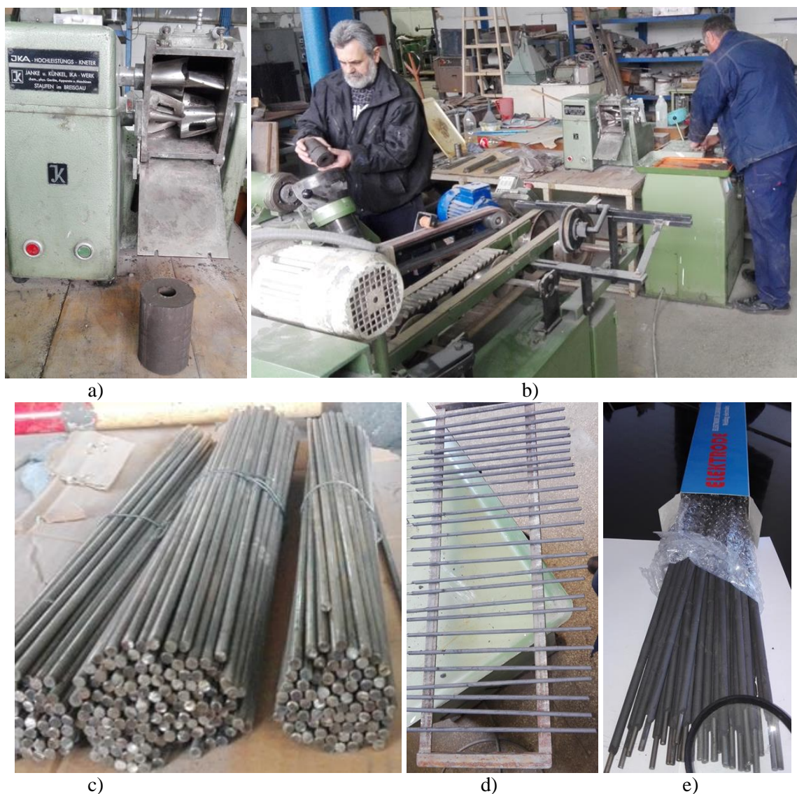
Figure 1. A W-mixer for wet mixing of the coating mass (a), experimental electrode coating (b), preparing of metal core, a rod 4 mm in diameter and a length of 350 mm (c), the electrodes, after drying, (c) and samples of the electrodes after drying and packaging (d, e)
