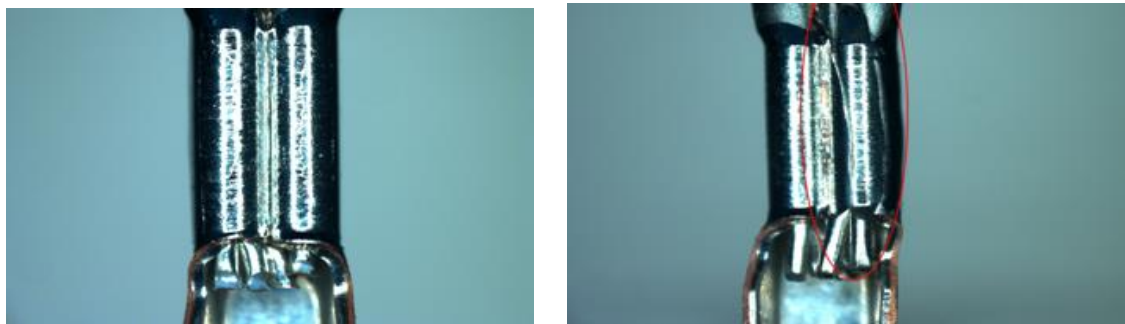
Figure 5. “Correctly crimped connector (left) and incorrectly crimped connector (right)”
