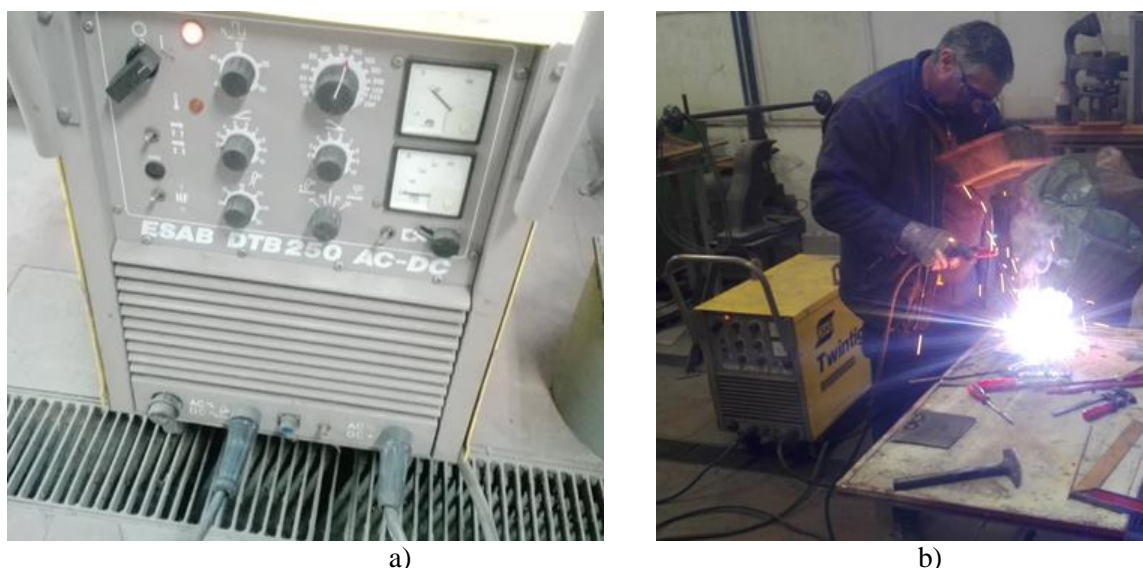
Figure 2. The ESAB DTB 250 AC-DC device for experimental MMA- process welding with a new electrode
