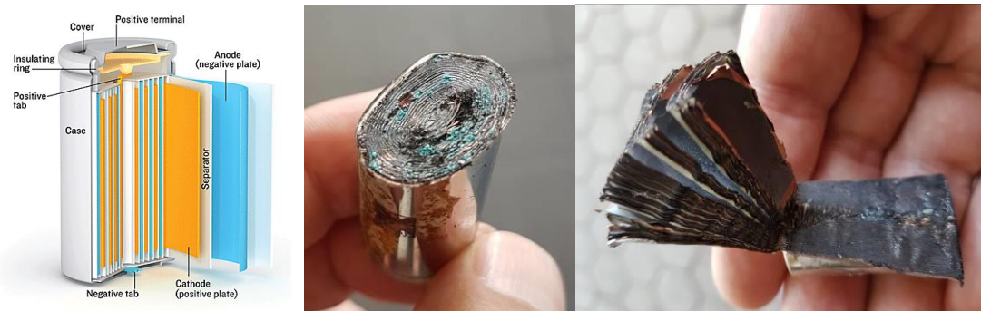
Figure 5. Construction and interior design of a 18650 cylindrical battery
