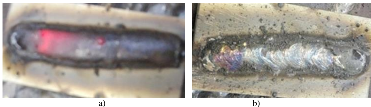
Figure 4. Experimental surfacing of AISI 304 stainless steel using MMA-process with the basic electrode
