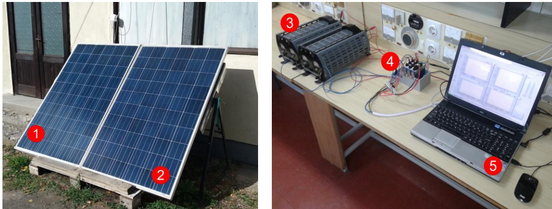
Figure 1. Testing PVT and PV modules and data acquisition system 1 – hybrid PVT solar collector, 2 – PV solar collector, 3 – resistor, 4 - acquisition cards, 5 - computer
