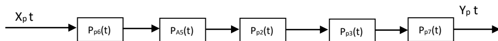
Figure 4. Reduction of a block diagram in the III step for the circuit of the spinning box
