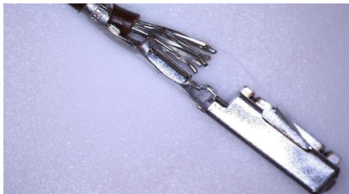
Figure 3. “Wires outside the crimp”
