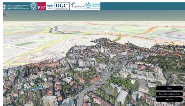
Figure 2. 3D point cloud for the city of Novi Sad
