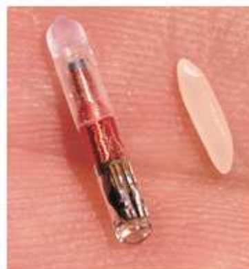
Picture 6. VeriChip compared to a grain of rice
