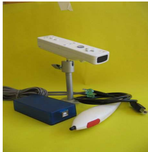
Picture 5. The Wii control and the infrared pen with the accessories
